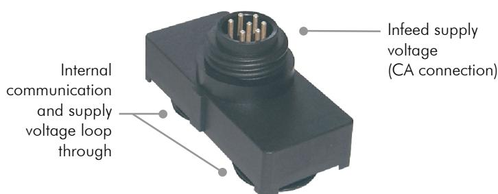
The infeed module feeds the supply voltage for the bus coupler module and the sensors and actuators via a CA connection. It connects the bus coupler module to the first I/O module or connects two I/O modules.
