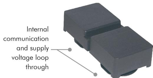
The bridge module connects two I/O modules and serves to transmit internal communication and loop through the supply voltage for sensors and actuators.
